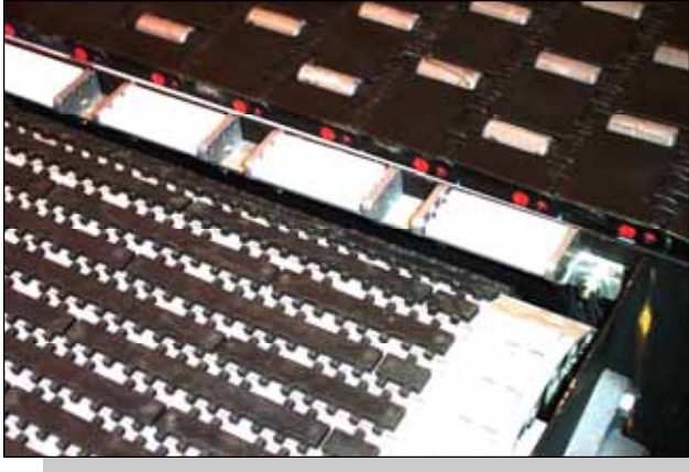
Single roller modules used to transfer product from Rex® 3004 MatTop® chain to Rex® 7705 RubberTop™ MatTop® chain .
