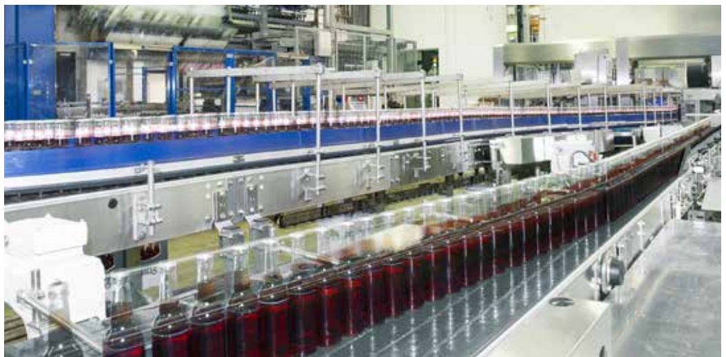
High-speed glass bottle filling line, equipped with Rexnord TableTop chain.
