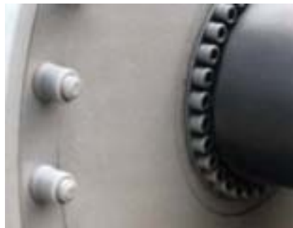
Segmental-rim sprockets and traction wheels simplifies installation and replacement. Keyless locking ring holds wheel to shaft.
