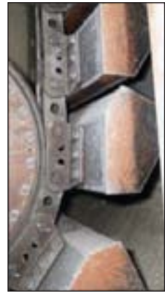
Rexnord internal gravity take-up assembly provides constant tension on the elevator chain and automatically adjusts tension to allow for chain elongation.
