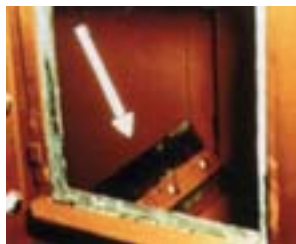
Adjustable rubber peeler lip at the discharge chute picks up slow or late discharging material and helps prevent this material from falling into the boot section. Standard on both belt and chain bucket elevators.
