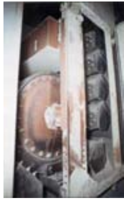
Rexnord® 900 Series Elevator Chains wrap around a segmental traction wheel. All components receive special heat treatment for extended wear life.
