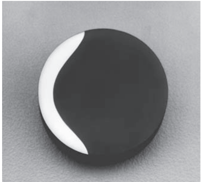
A cross section of a selectively induction hardened WHX pin - the crescent area is super-hardened to dramatically lengthen pin wear life. The balance of the pin material is left in the thru-hardened condition to give the pin excellent toughness.
